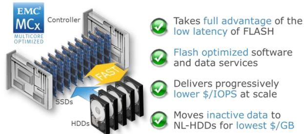
In addition, VNX-F all-flash configurations deliver consistent performance and low latency for application environments that require the lowest \$/IOPS. MCx (Multi-Core RAID, Multi-Core Cache and Multi-Core FAST Cache) distributes all VNX data services across all Cores – up to 32. This approach delivers unprecedented application performance while maintaining affordable pricing: Compared to the previous generation, the VNX series with MCx delivers:
